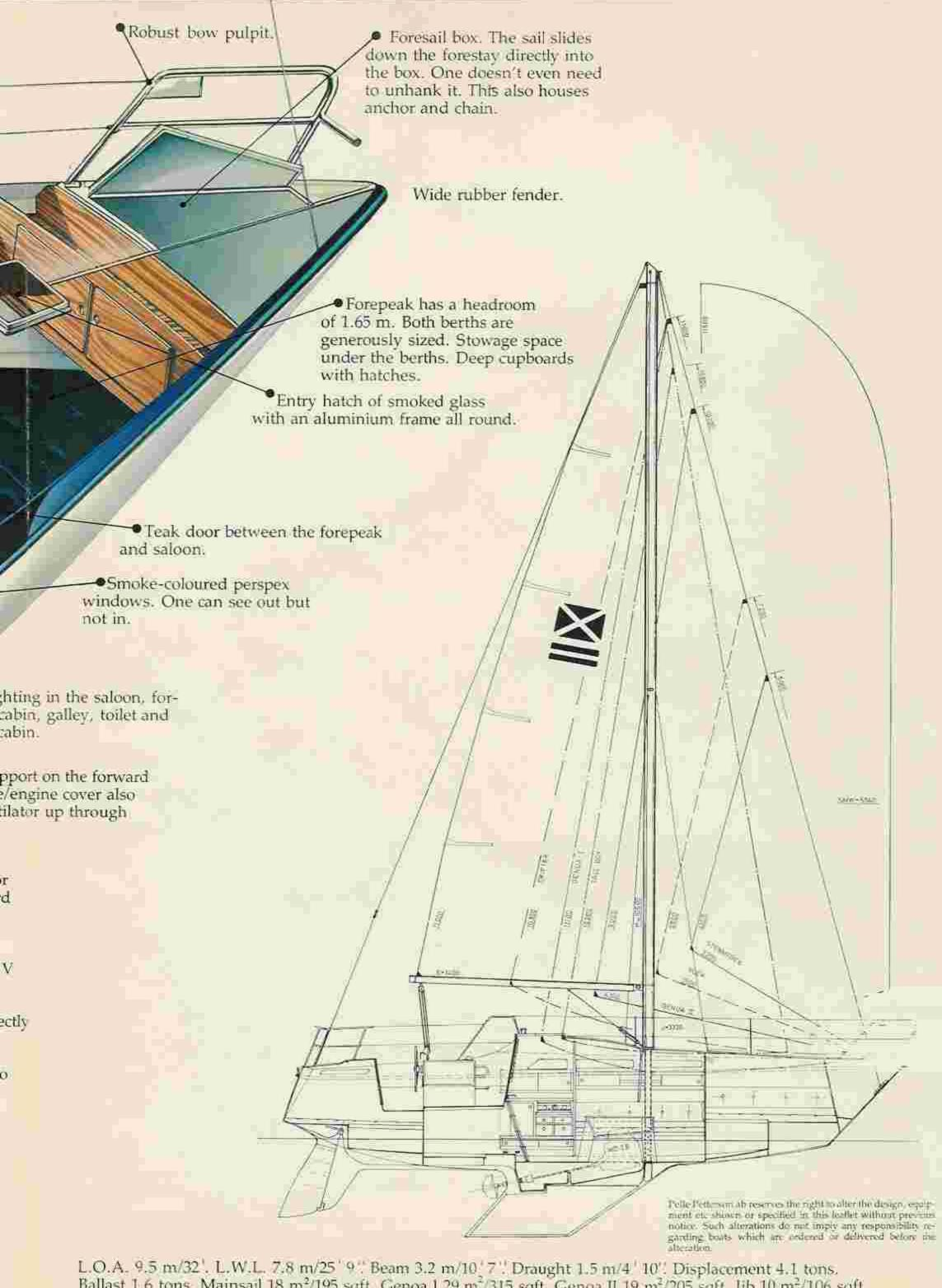
L.O.A. 9.5 m/32<sup>1</sup>. L.W.L. 7.8 m/25<sup>1</sup> 9." Beam 3.2 m/10<sup>1</sup> 7." Draught 1.5 m/4<sup>1</sup> 10". Displacement 4.1 tons. Ballast 1.6 tons. Mainsail 18 m<sup>2</sup>/195 sqft. Genoa 1 29 m<sup>2</sup>/315 sqft. Genoa II 19 m<sup>2</sup>/205 sqft. Jib 10 m<sup>2</sup>/106 sqft. Stormjib 7 m<sup>2</sup>/75 sqft. Spinnaker 70 m<sup>2</sup>/755 sqft.
